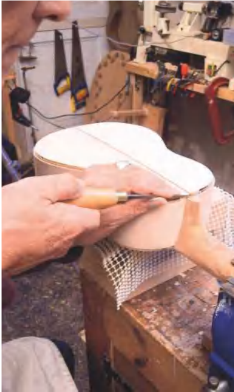
STEP 38. Chiselling the slots
